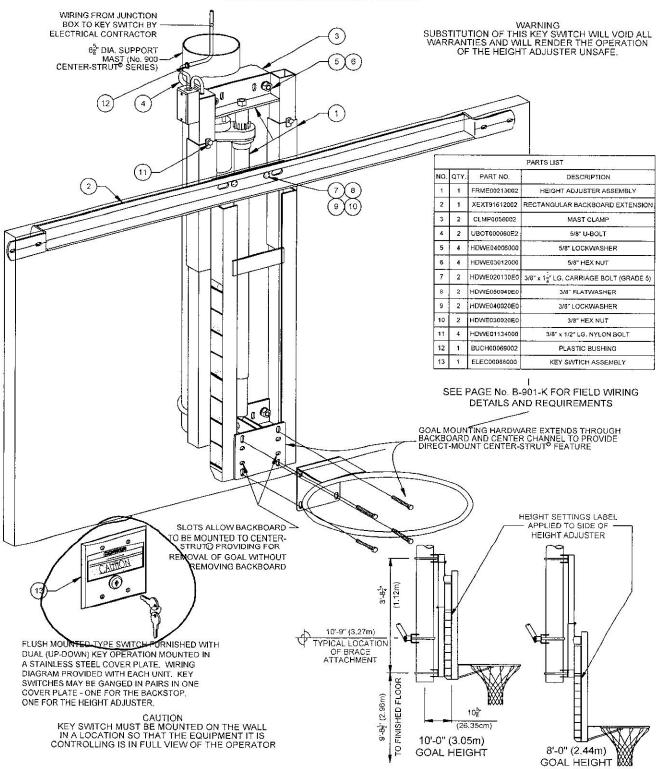
\_\_\_ - 00901506 KEY SWITCH OPERATION FOR RECTANGULAR BACKBOARD SEE B-200 FOR BACKBOARD AND GOAL OPTIONS
