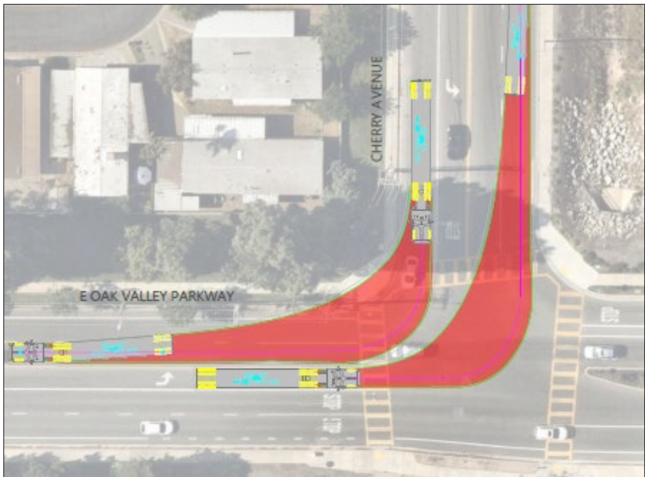
Figure 15. WB-67 Truck Turning Movements – E Oak Valley Parkway and Cherry Avenue
