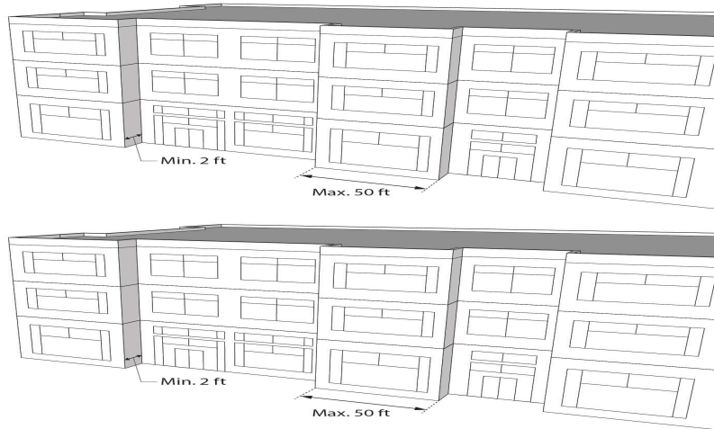
Figure 17.19-3. Wall Plane Modulation
