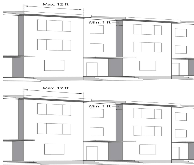
Figure 17.03-11. Required Facade Articulation
