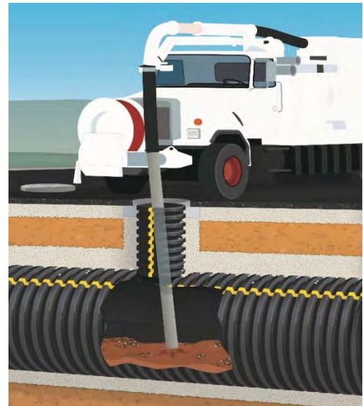
Figure 3: Vacuum Truck Removing Sediment and Debris
